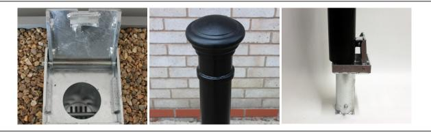
a traditionally styled ornamental bollard designed to resemble its cast iron relative. The body of the bollard is manufactured from mild steel which is galvanised as standard to ensure its longevity. Caps and rings manufactured from cast iron are welded on to the steel body to complete the design.
